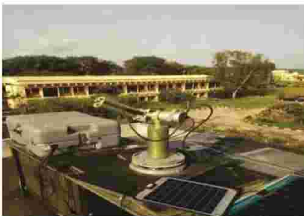
Figure 2 AERONET CIMEL Sun-photometer at block 9 of the faculty of physical science, University of Ilorin, Nigeria.
